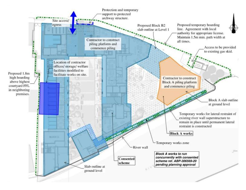
Figure 4.3 Overall sequencing of Works (2 of 7)
