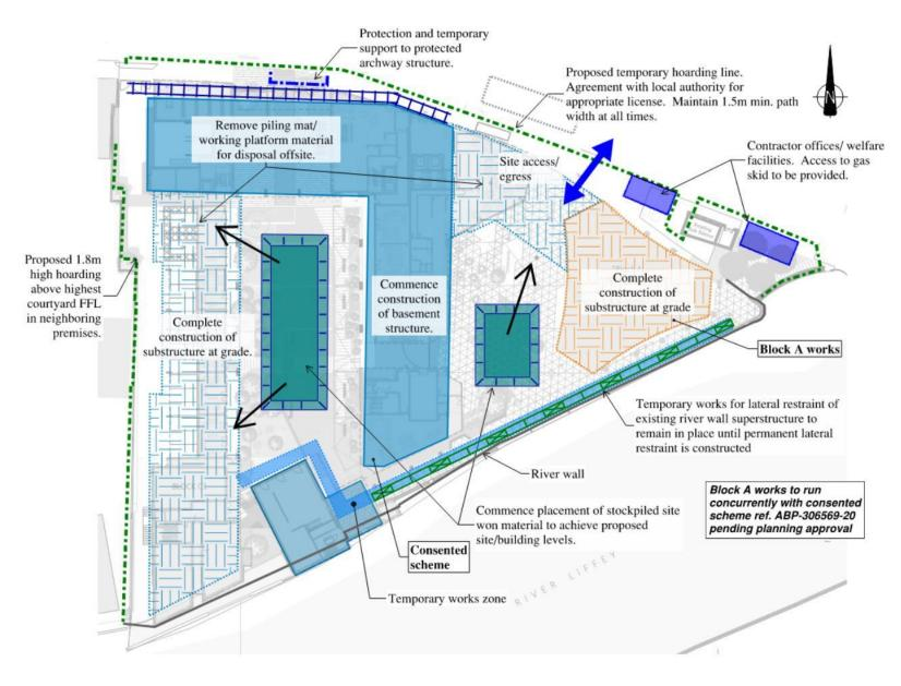
Figure 4.5 Overall sequencing of Works (4 of 7)
