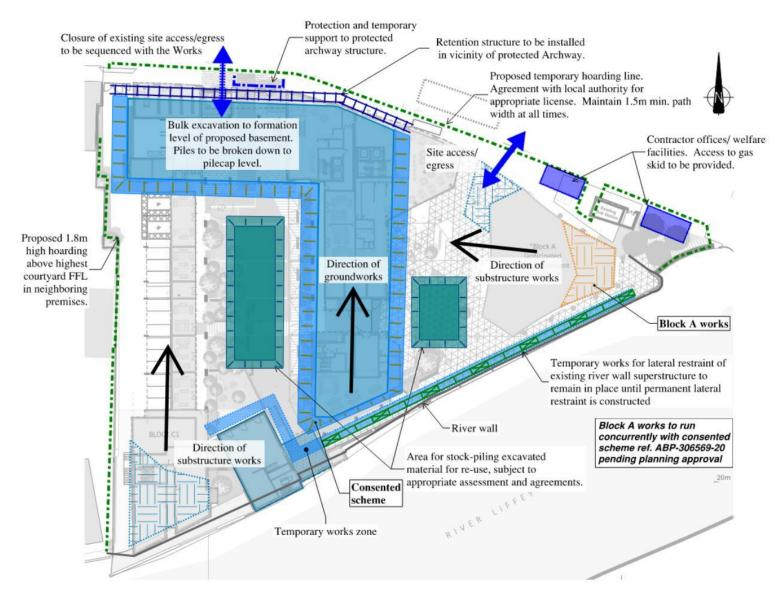
Figure 4.4 Overall sequencing of Works (3 of 7)
